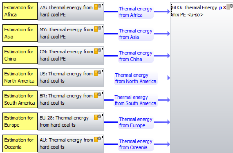
Figure 11: GaBi plan for thermal energy modelling from hard coal in the global model
