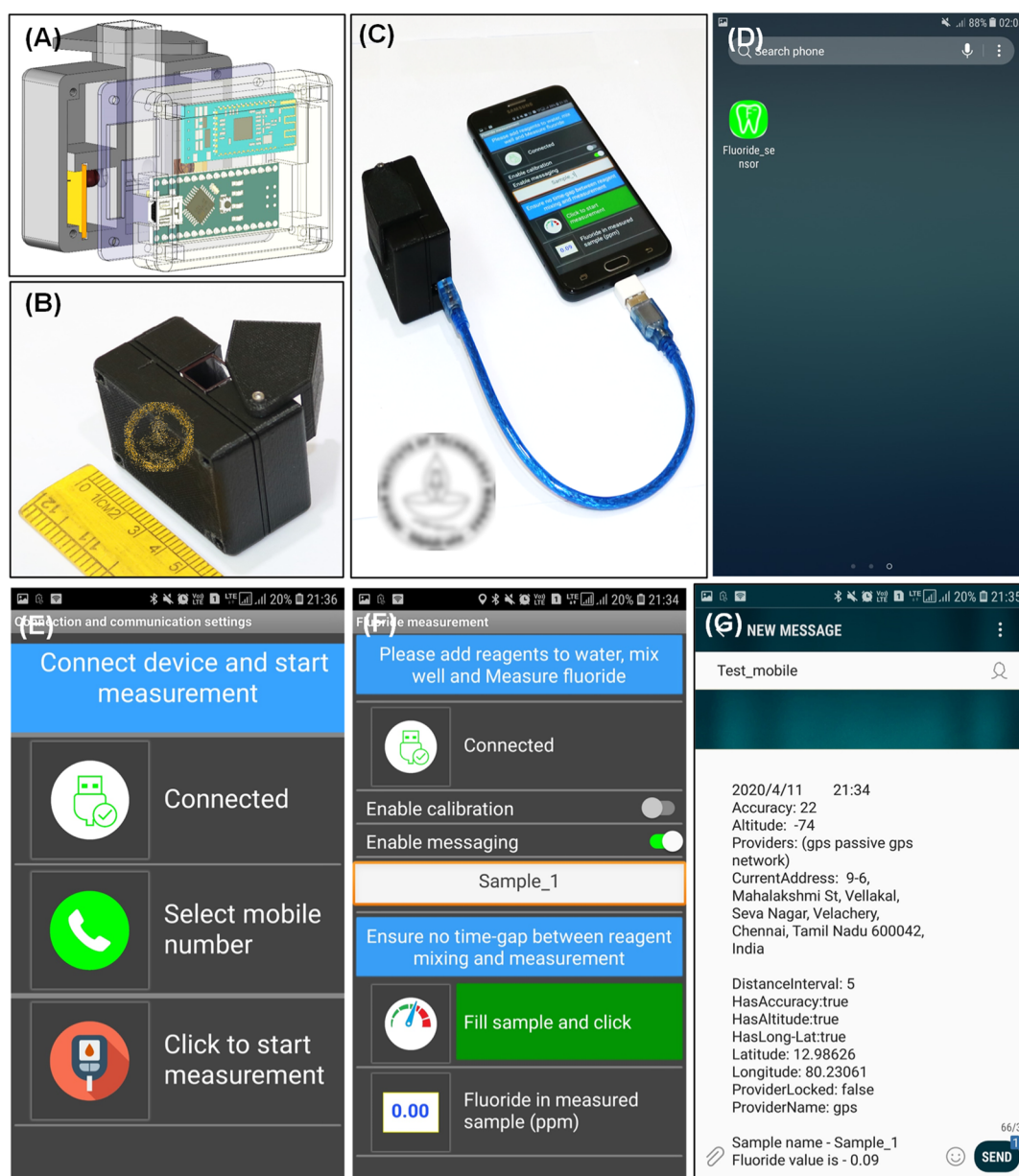
Figure 6. (A) Graphical representation of the extended sensor device cum sample holder. (B) Photograph of the sensor extension cum sample holder. (C) Photograph of the F^- sensor integrated with a smartphone. (D) Icon of the customized mobile application developed for the F^- sensor. (E,F) Screenshot images of the application of a precalibrated sensor for the detection process and for real-time data sharing and storage; and (G) final screen containing the result and the details related to the sample.
