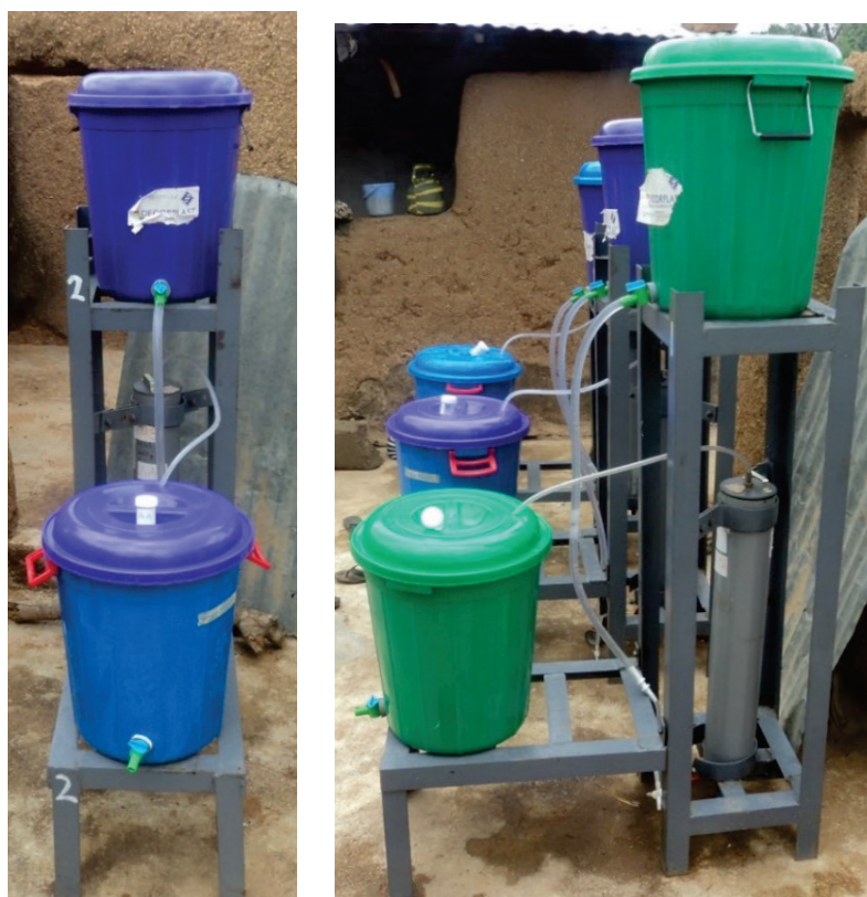
Fig. 6.2 Pilot-scale household defluoridation units at Bongo, Upper East region of Ghana, filled with AFWC, RAFWC and AA.
