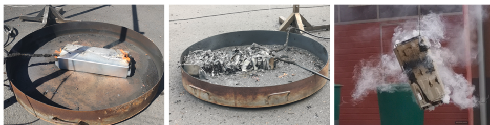
Fig. 1. Vehicle batteries after ignition (before submerging into the barrel with water). Left – module A (ignited by short circuit, visible but small fire, no blasts), Middle – module B (ignited by repeated breakthrough, complete destruction, heavy fire, several blasts), Right – module C (heated by hot plate and ignited by repeated breakthrough, without visible fire, only white smoke release).
