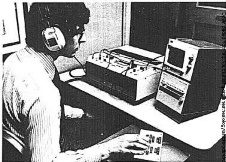
FIG. 1. Volunteer seated at audiovisual test described in text. The tape recorder is sending auditory signals to the earphones and visual signals to the two-channel oscilloscope. The subject indicates recognition of a change in either mode by depressing the appropriate button on the response panel.
