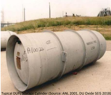
Typical DUF<sub>6</sub> Storage Cylinder (Source: ANL 2001, DU Oxide SEIS 2018)
