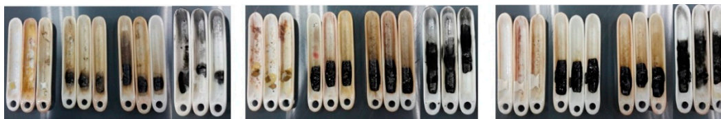
Figure 5. Pictures of pyrolysis char residues of each sample at 300 °C, 400 °C, 500 °C, and 900 °C for the three sample types PPE, TPT, and KPK (from left to right).
